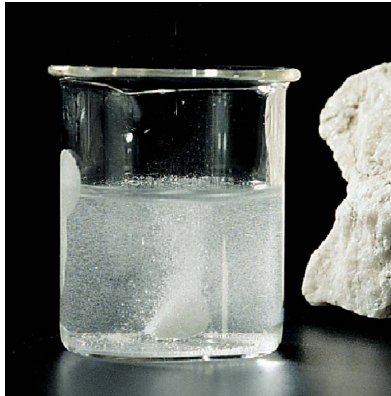
Figure 19.13 Test for the presence of a carbonate.
