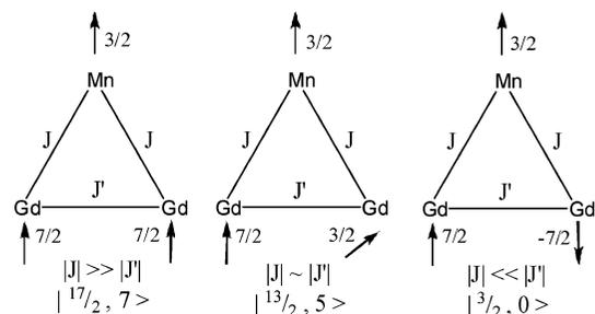
**Figure 4.** Depictions of the indicated  $|S_T, S_A\rangle$  states, showing (left) the complete frustration of  $J'$  and the resultant  $S_T = 17/2$  ground state, (middle) the intermediate situation, giving the  $S = 13/2$  ground state of **1**, and (right) the complete frustration of  $J$  and the resultant  $S_T = 3/2$  ground state.
