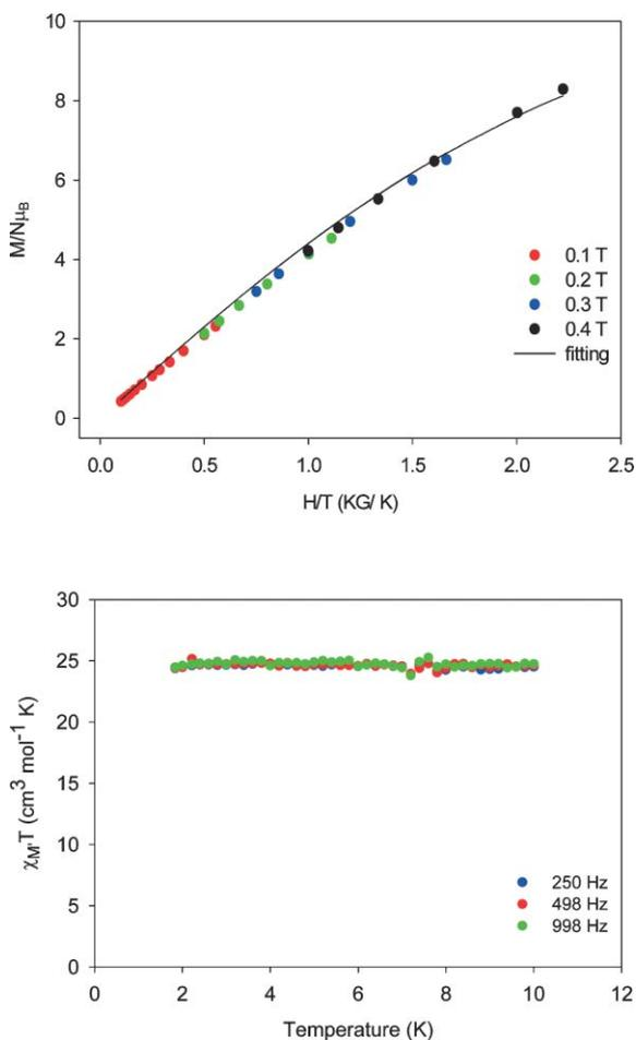
Fig. 5 Reduced magnetization data (top) and ac magnetic susceptibility data (bottom) for complex **2**.
