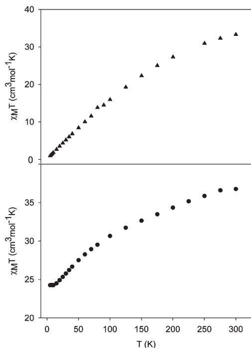
Fig. 4 Plot of  $\chi_M T$  vs.  $T$  for complexes **1** (top) and **2** (bottom).
