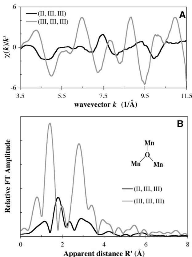
**Fig. 7** Mn EXAFS (A)  $k$ -space (weighed by  $k^3$ ) and (B) its Fourier transform for each of the Mn<sub>3</sub>O compounds.
