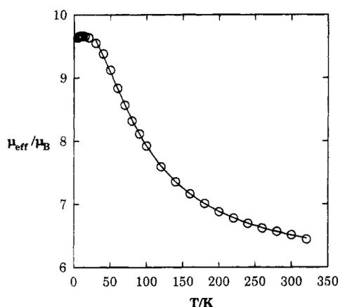
**Figure 5.** Plot of  $\mu_{\text{eff}}$  versus  $T$  for [Ni<sub>4</sub>(N<sub>3</sub>)<sub>4</sub>(dbm)<sub>4</sub>(EtOH)<sub>4</sub>] (3). The solid line represents the fit to a one- $J$  model; see the text for fitting parameters.
