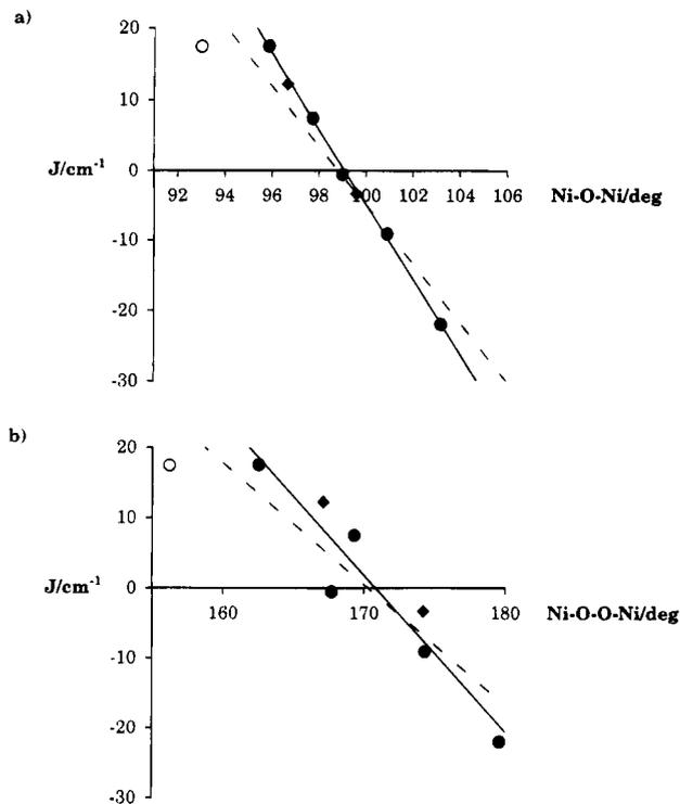
**Figure 6.** Effect of (a) average Ni–O–Ni angle and (b) average Ni–O–O–Ni torsion angle on  $J$  for  $[\text{Ni}_4(\text{OR})_4]^{4+}$  cubanes: (●) literature data (refs 10, 12, 13, 14); (◆) this work. Dashed lines represent lines of best fit for all data; solid lines, for data omitting one interaction (○) involving an additional acetate bridge (ref 13; see text, Table 6).
