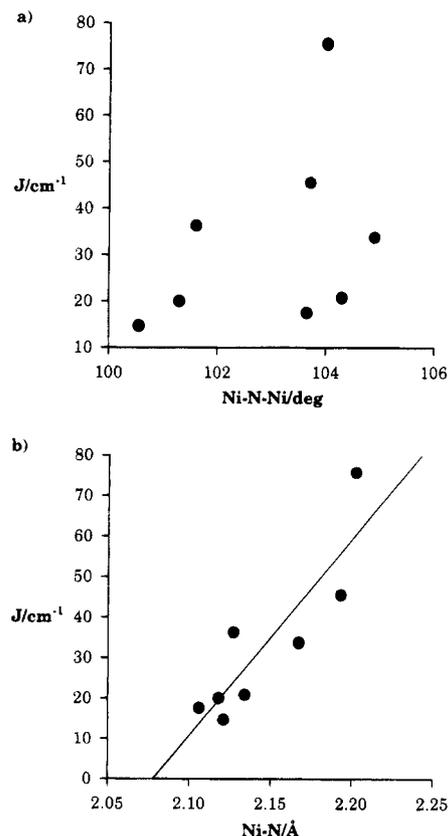
**Figure 8.** Effect of (a) the average Ni–N–Ni angle and (b) the average Ni-( $\mu\text{-N}$ ) distance on  $J$  for dimeric and polymeric Ni<sup>II</sup> complexes containing the planar  $[\text{Ni}_2(\eta^1, \mu\text{-N}_3)_2]^{2+}$  bridging motif.
